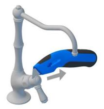
Remove the handle from the cartridge spline.
