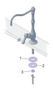
Under the wash basin, tighten the nut using a suitable spanner or shifter.
