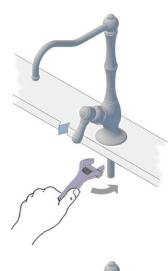
Securely fit the ½" adaptor 4, to the end of the threaded section.
