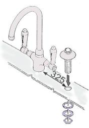
Insert the hand spray escutcheon into the sink hole.
