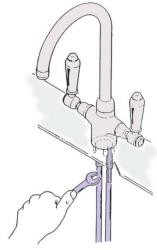
Check the position on the sink of the tap, then tighten the nut using a 13mm wrench.
