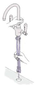
Insert the tap into mounting hole. Feed the water supply hoses carefully through the hole ensuring that they are not bent or kinked, as this could result in permanent damage or leakage.
