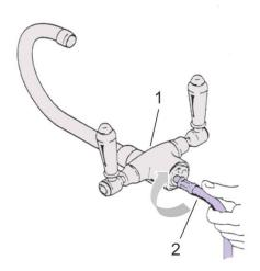
Install the water supply hoses into the body - 1
