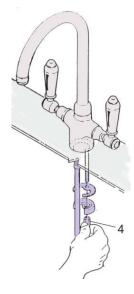
Under the sink, stack the supplied half ring rubber gasket above the half ring mounting plate feed them onto the stud. Then screw the mounting nut -4, onto the stud. Screw the mounting stud until the half ring rubber mates up with the underside of the sink.
