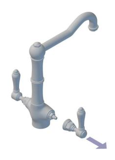
**NOTE**: At any time, should the handle feel loose, retighten the retaining flange.
