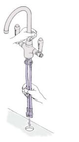
Insert the tap into mounting hole. Feed the water supply hoses carefully through the hole ensuring that they are not bent or kinked, as this could result in permanent damage or leakage.
