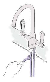
Check the position on the sink of the tap, then tighten the nut using a 13mm wrench.
