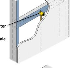
Install the connector pipe 1, into the wall elbow connector. Ensure that the pipe is adequately sealed using PTFE tape or appropriate sealing material to ensure a water tight connection.
