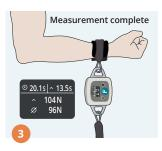
The measurement will stop once the client stops producing force or when the button is pressed once more.
