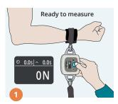
Press the measurement button to enter measurement mode
