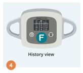
Press the measurement button one last time to return to the history view where the last four measurements are shown.
