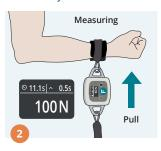
Start the measurement by either pressing the button again or by having the client produce force.
