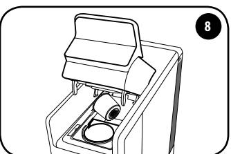
To eject the used capsule, slowly lift the lever and the capsule will be automatically collected in the specific container. If the capsule is not ejected, repeat the operation.
