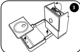
Empty the capsule holder and rinse it. Clean the tray and grid of residual water and coffee. Once clean, engage the tray in the grid.
