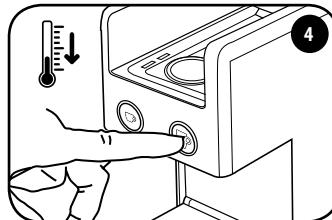
Press the button ☕ to decrease the temperature. The ☕ button flashes. Both buttons flash after approx. 3 seconds.
