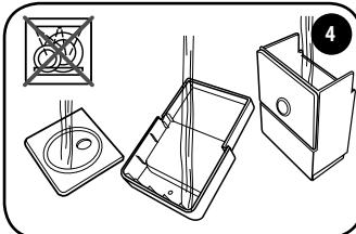
Rinse the components under running water and dry them. Do not wash the components in the dishwasher.
