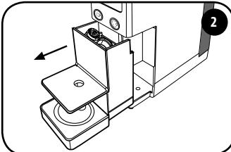
Remove the capsule holder. The capsule holder can contain a maximum of 7 capsules. Therefore it should be emptied regularly to prevent the capsules from getting stuck.
