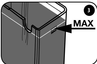
Fill the tank with fresh water to the maximum level.
