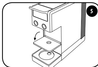
Lower the cup support grid. Fill the tank with fresh drinking water.
