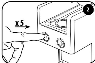
Press the ☕ button 5 times within 15 seconds of turning on the machine. Both buttons will flash. It is now possible to change the temperature as described in points 3 and 4.
