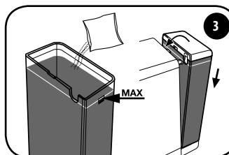
Fill the tank with fresh water to the maximum level and let the descaling solution dissolve.
