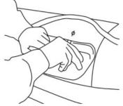
Attach the oarlock to the inflatable boat and make sure that no air bubbles are left between the pad and the boat. After the pad is set in place and all the air bubbles are out from under the oarlock, let it sit for 48 hours. Do not touch until the glue has properly set.
