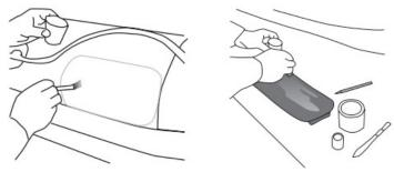
Let the glue set until the surface is no longer tacky to the touch (approximately 10-15 mins). Next spread a 2<sup>nd</sup> thin layer of glue to both the oarlock pad and boat and let it set again until tacky. We recommend then using a hair dyer to warm the surface of the pad and boat. Once warm (not hot) to touch stick the pad to the boat.
