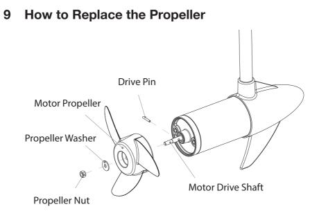
**A WARNING** Make sure that the motor has been disconnected from batteries before handling the propeller.
