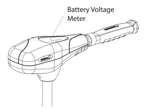
When the motor is connected to the battery, the battery meter will light up to indicate the amount of power left in the battery. There are 5 LED lights on the top cover, when four (4) blue LED's are out, the meter is indicating that the input voltage is less than 9.5V (normal voltage draw, 12V). It is advised to disconnect the motor from the bat- tery to prevent damage to the battery and recharge.
