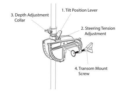
**WARNING** Before the installation, make sure the area between column and bracket is clear.
