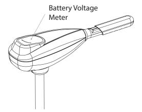
When the motor is connected to the battery, the battery meter will light up to indicate the amount of power left in the battery. There are ten LED lights on the top cover. When seven LED's are out, the meter is indicating that the input voltage is less than 9.5V (normal voltage draw is 12V). At this point it is advised to disconnect the motor from the battery to prevent damage to the battery and recharge.
