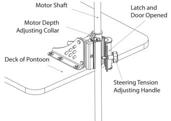
Close the latch and door and tighten the steering tension adjusting handle, making sure the motor assembly is in place properly.
