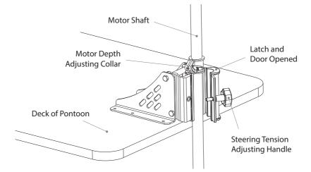
Close the latch and door on the mounting bracket and loosely tighten the steering tension adjusting handle. Place the motor aside.
