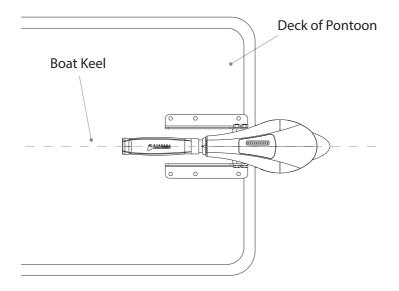
We recommend installing the motor along the centerline or keel of the pontoon boat. Before the installation, remove the motor assembly first and place the mounting bracket at the desired position.
