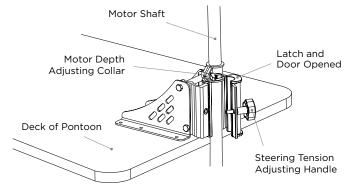
Closing the latch and door on the mounting bracket and loosely tighten the steering tension adjusting handle. Place the motor aside.
