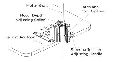
Close the latch and door and tighten the steering tension adjusting handle, making sure the motor assembly is in place properly.
