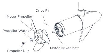
**MARNING:** Make sure that the motor has been disconnected from batteries before handling the propeller.
