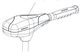
When the motor is connected to the battery, the battery meter will light up to indicate the amount of power left in the battery. There are 5 LED lights on the top cover, when four (4) LED's are out, the meter is indicating that the input voltage is less than 9.5V (normal voltage draw, 12V). It is advised to disconnect the motor from the battery to prevent damage to the battery and recharge.
