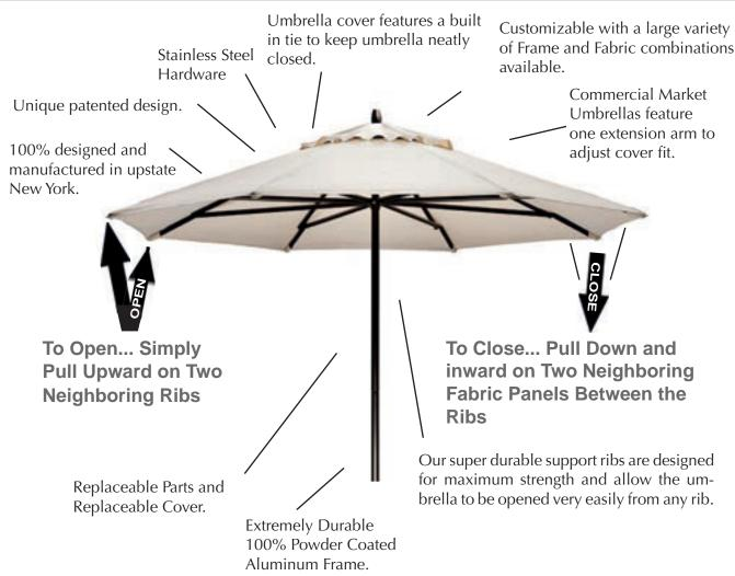
Simple yet effective, our unique and patented (US 8,230,869 / 8,302,616) mechanisms allow you to raise and lower your umbrella by simply pulling on the ribs or pushing on the fabric. This design is especially helpful with the use of larger dining tables where access to the umbrella crank is limited. It also adds to the durability and aesthetics of the umbrella.
