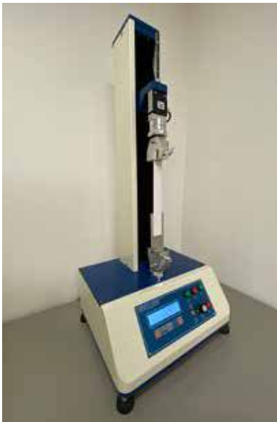
IN-HOUSE TENSILE AND ADHESION TESTING FOLLOWING ASTM STANDARDS.
