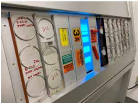
IN-HOUSE UV/CONDENSATION TESTING PER ASTM STANDARDS
