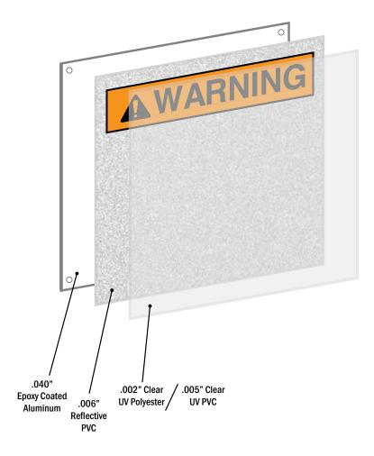
CM300 Reflective/Aluminum Signs are great medium duty indoor/outdoor signs. Signs feature durable UV inks printed on Engineer Grade retro-reflective sheeting with a thick .040" aluminum base layer. All signs are laminated with an overlaminate that sheds UV, moisture, chemicals and abrasion. Available with holes or adhesive back.
