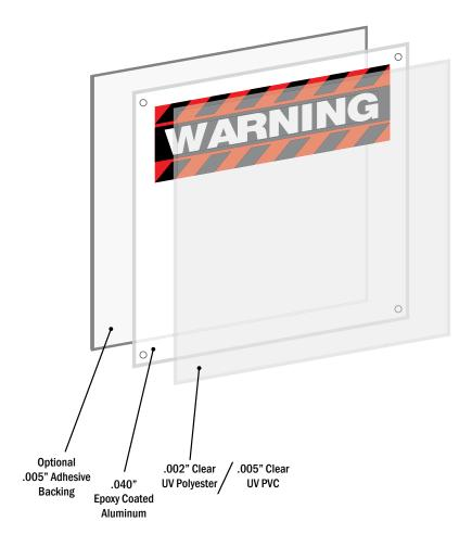
CM200 Aluminum Signs are great medium weight indoor/outdoor signs. Signs feature UV inks that hold up very well outdoors. All signs are laminated with an overlaminate that sheds UV, moisture and abrasion. Specify polyester overlam if subjected to chemicals. Available with holes or adhesive backs.
