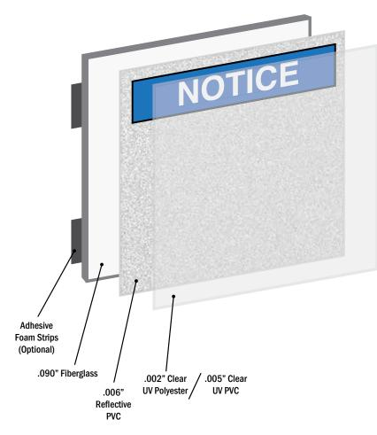
CM175 Reflective/Fiberglass Signs are great heavy duty indoor/outdoor signs. Signs feature durable UV inks printed on Engineer Grade retroreflective sheeting with a thick .090" fiberglass base layer. All signs are laminated with an overlaminate that sheds UV, moisture and abrasion. Specify polyester overlam if subjected to chemicals. Available with holes or adhesive backs.
