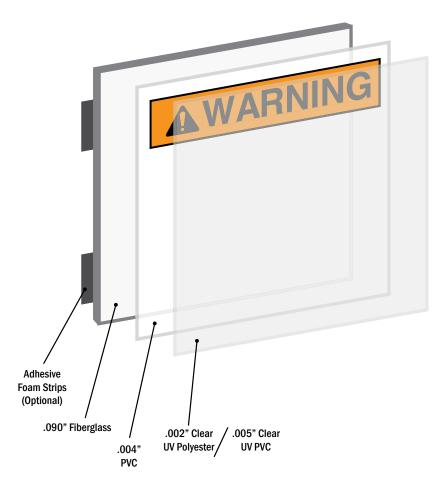
CM125 PVC/Fiberglass Signs are great heavy duty indoor/outdoor signs. Signs feature durable UV inks printed on durable .004" PVC (vinyl) sheeting with a thick .090" Fiberglass base layer. All signs are laminated with an overlaminate that sheds UV, moisture and abrasion. Specify polyester overlam if subjected to chemicals. Available with holes or adhesive backs.
