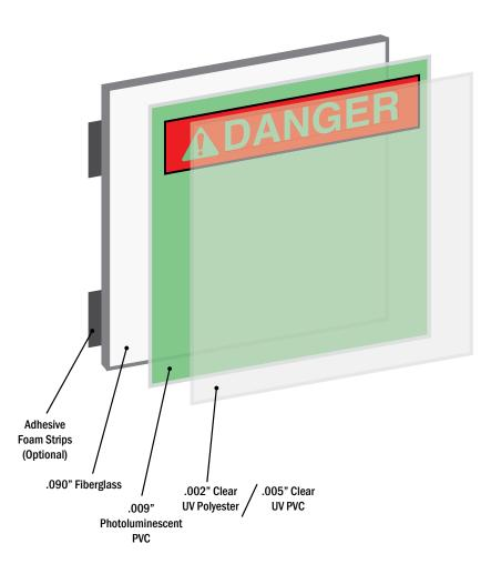
CM100 Photoluminescent/Fiberglass Signs are great heavy duty indoor/outdoor signs. Signs feature durable UV inks that hold up very well outdoors. The luminescent material gathers light and then emits it in total darkness for up to 8 hours. All signs are laminated with an overlaminate that sheds UV, moisture, chemicals and abrasion. Available with holes or adhesive back
