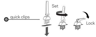
Place mounting bracket in center and align quick clip holes.
