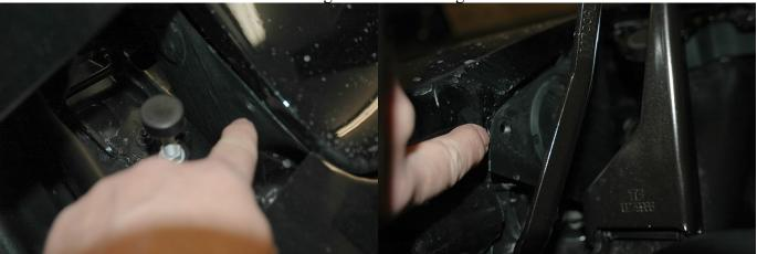
4. Remove the cover from the manual screws on both headlight motors and turned them to raise the headlight assemblies to their highest point. Pull up on the front of the headlight while raising it manually to make it easier to turn
