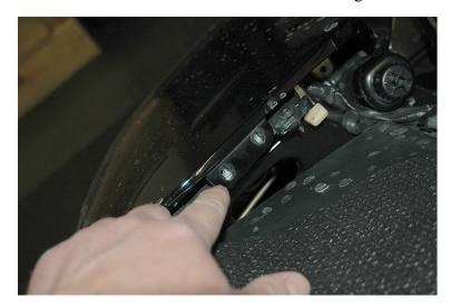
3.Remove two accessible screws to the headlight shrouds with lights still down
