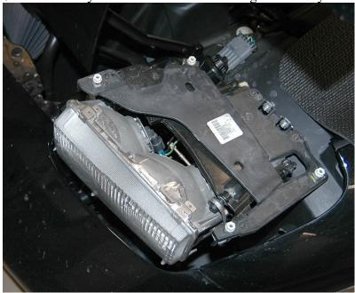
9. There are two bushed shoulder bolts held on with thread locked nuts that need to come out. Use WD-40 to help with removal. Be extremely careful unscrewing the bolts so you don't strip or break them. Keep the shoulder screw, bushing, and nut in a safe place\_
