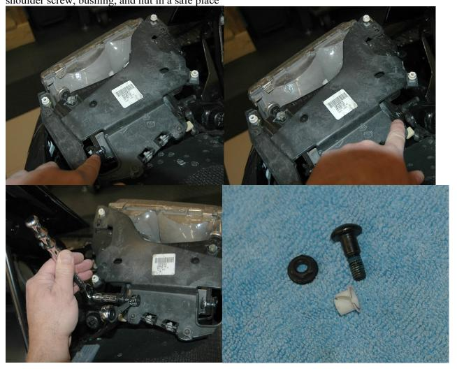
10. Once the rear hinges are free, flip the headlights forward from the back, remove the electrical connectors from the rear of the lamp housings and expose the underside where there is a pin about 3/8" in diameter with a retaining washer that needs to be popped off so the pin can be extracted. This pin runs through the pivot bracket that is attached to the gear motor that raises the headlight. The yellow arrow points to the pivot bracket in the picture below
