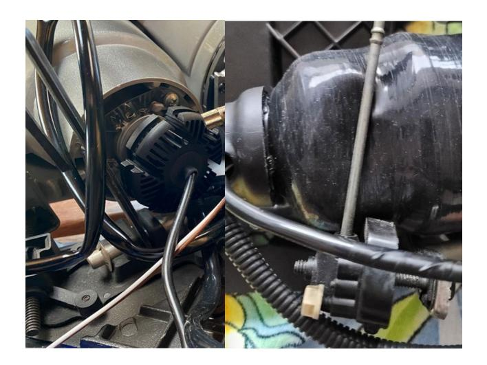
14. Then place the headlight assemblies in the compartment loosely, taking care to wrap/tape the lenses for protection. Push the harness connectors into the appropriate receivers and connect the OEM headlight connectors to the correct connectors on the housings taking care to match the positive/negative.
