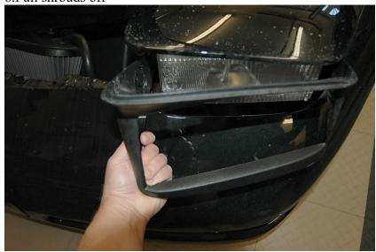
7.Remove the two side screws from each of the headlight covers.
