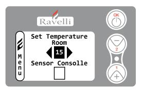
To modify the thermostat value press Key 1. Enter the Set Temperature menu and with Keys 1 and 2 set the desired room temperature at which the fire will enter Modulation Work Mode.
