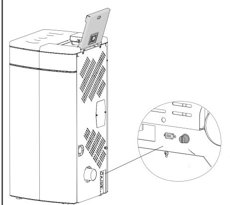
Unscrew the protection cap and press the button to reset the thermostat alarm.
