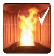
The combustion IS CORRECT, full flame yellow/white and minimum quantity of pellet in the firepot.
