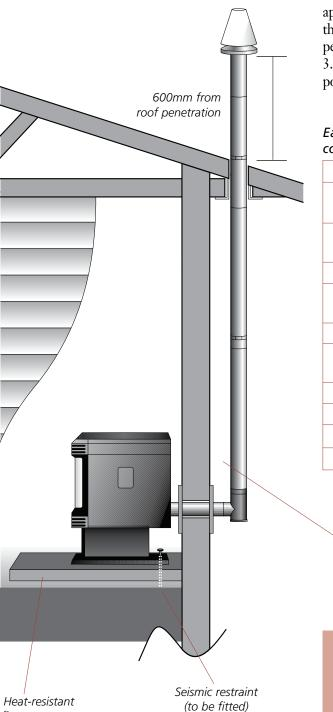
This flue kit may be used in new and replacement applications with the flue penetrating the wall behind the fire, running vertically up an outside wall and penetrating the soffit. The overall height of the flue is 3.6m. All visible flue has a galvanised finish, and can be powdercoated on request. Kit is supplied in a carton.
