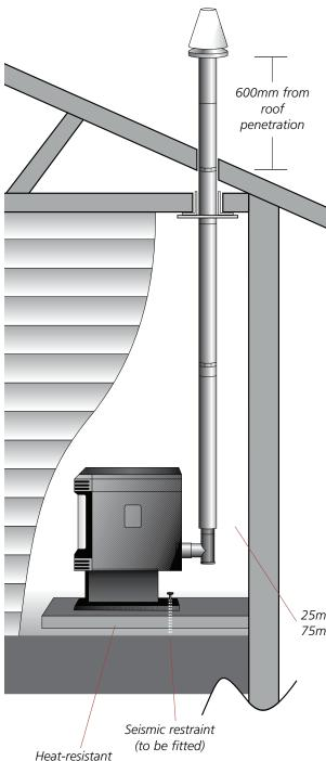
This flue kit may be used in new and replacement applications in rooms with stud height of 2.4m. The overall height of the flue is 3.6m. The visible flue is finished in black and the ceiling plate is white. The support angles for securing the liner to the ceiling are not shown. Kit is supplied in a carton.
