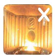
INCORRECT combustion - the flame is weak and there are a lot of unburned pellets in the firepot. Check first that the ash pan is properly closed. Then adjust set pellet/air increasing the air percentage (from 0 up to +5). If this doesn't work, try increasing the loading quantity of the pellet (from 0 up to -5) to reach the flame condition shown in picture 3.
