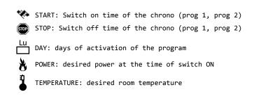
With the function chronothermostat it is possible to program for each day of the week the switch on and off of the stove in four independent intervals time (PROGAM 1, PROGRAM 2, PROGRAM 3, PROGRAM 4).
