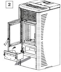
HOW TO REMOVE THE FLAME TRAP:
