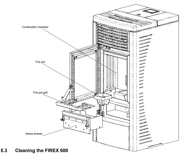
All Ravelli products have a combustion chamber made with FIREX 600, a material based on vermiculite, the result of research and development by Ravelli. The main features of FIREX 600 is its resistant to heat, its lightness and its excellent insulating capacities, which improve the combustion and performance of the stove. During combustion, FIREX 600 turns white, due to an effect called PYROLYSIS, making the flame clear and shining. If the combustion is regulated in an optimal way, the
