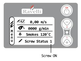
To return to the main screen press keys 1 and 2 at the same time. Repeat the operation several times until you see the pellets fall into the firepot. It is possible to do this operation only if the stove is in FINAL CLEANING phase or OFF.
