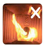
The combustion is NOT CORRECT, the flame is weak and a lot of unburned pellet wood into the firepot. Check first that the ash pan is properly closed. Then adjust set pellet/air increasing the air percentage (from 0 up to +5); in the event this is not enough, increase the loading quantity of the pellet (from 0 up to -5) to reach the flame condition shown in picture 3.
