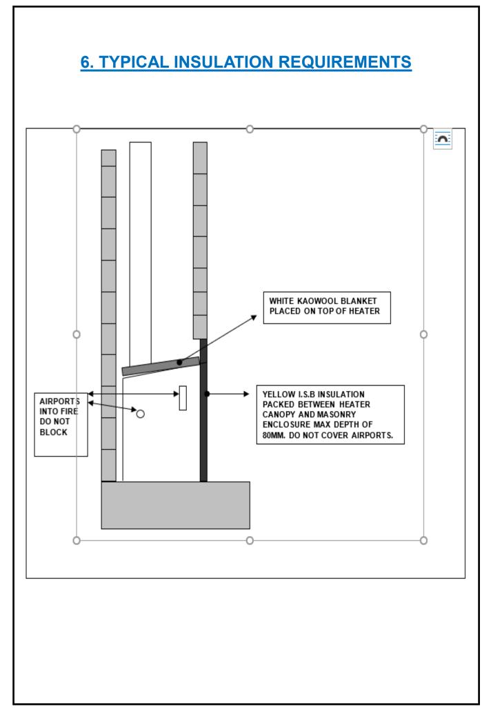
As this fire sources its combustion air from the chimney cavity, the fire <u>must be sealed</u> <u>using the yellow ISB insulation provided</u> around the front of the casing and masonry enclosure at the FRONT ONLY to a maximum depth of 80mm.
