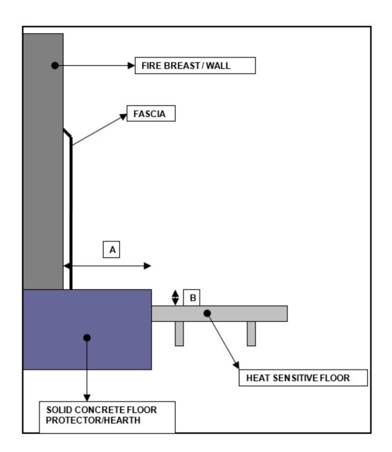
If the Fire is to be installed onto a SOLID concrete floor protector (hearth) that has no heat sensitive materials in its construction it must meet the following **MINIMIUM** dimension as marked A & B from above.
