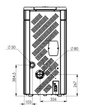
INSTALL VENT AT CLEARANCES SPECIFIED BY THE VENTING MANUFACTURER
