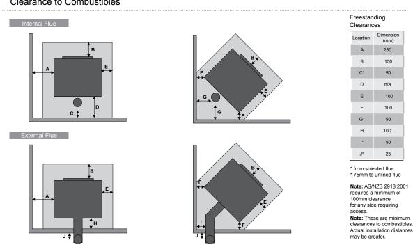
Note: The above clearance to combustibles on the flue are only applicable within the fire envelope. Clearance outside this e.g. at a ceiling / wall thimble reverts to 25mm as per ARS flue test 05/1185.
