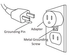
ground such as a properly grounded outlet box by a metal screw. The adapter should not be used if a three-slot grounded receptacle is available.
