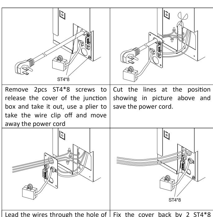
Lead the wires through the hole of the cover and connect with the wire from the fireplace by cables. Fix the cover back by 2 ST4\*8 screws.
