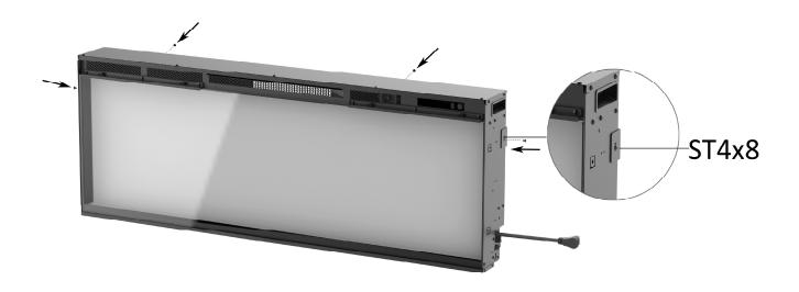
4a.5. Unscrew the glass fixing brackets and take the brackets and the glass out.
