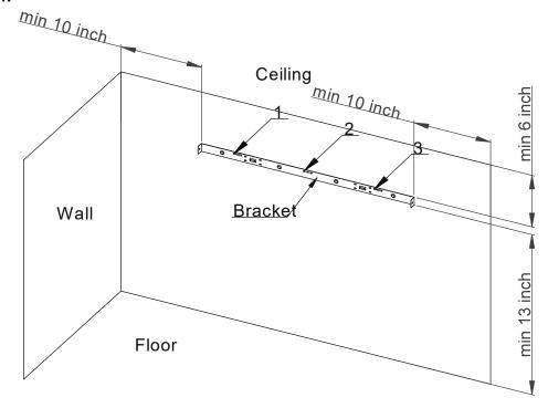
4b.3. Take away the bracket and drill 3pcs 40mm deep, Φ8 holes on the wall. Tap the plastic wall plugs into the holes. Secure the bracket by 3pcs ST5X40 screws.
