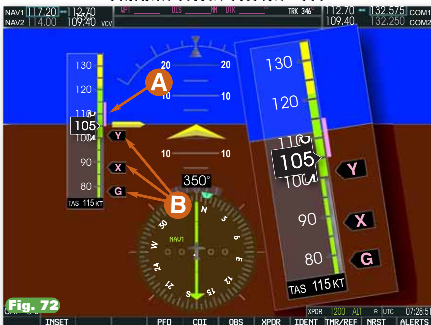
Fig. 72 The magenta trend line (position A) tells you what your airspeed will be in six seconds at the airplane's present pitch and power setting. Best rate, best angle and best glide speeds may also be shown by thumbnail identifiers (position B).
