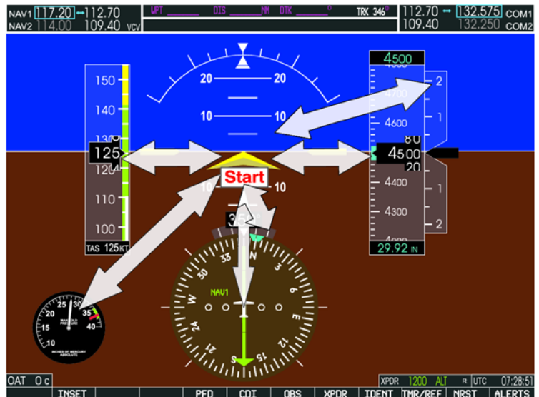
Figure 19. The instrument scan begins with the attitude indicator then moves to the primary instruments.
