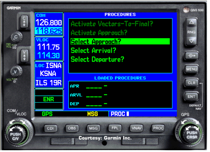
Figure 44. To load an instrument approach into your GPS, press PROC to open the "Procedures" window. Then highlight "Select Approach?" and press ENT.
