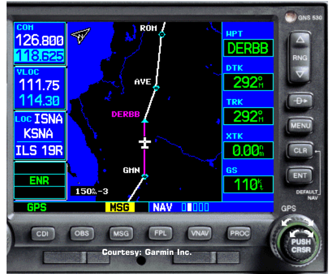
Figure 37. On Nav Page #2, you can see your new routing to San Jose airport.
