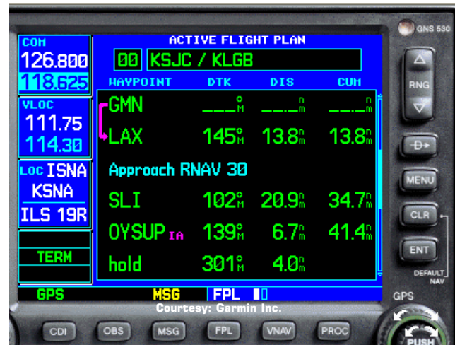
Figure 48. By "loading" the approach, its routing was appended to the end of your flight plan.
