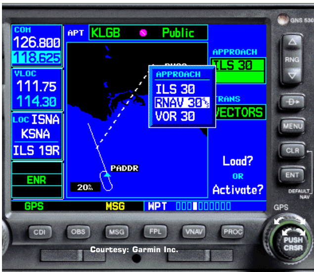
Figure 45. When the "Approach" box opens, move the cursor to RNAV 30 (GPS) and press ENT to select this approach.
