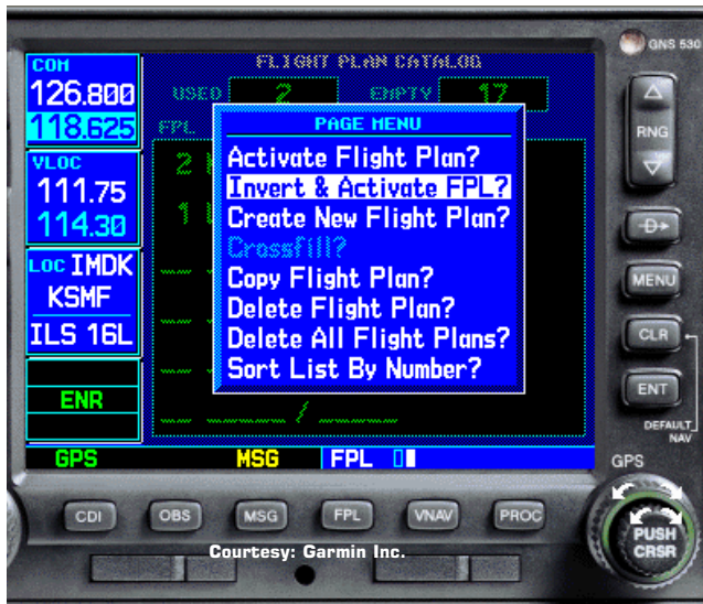
Figure 39. When the "Page Menu" opens, highlight "Invert & Activate FPL?" Press ENT which inverts and activates your return route.
