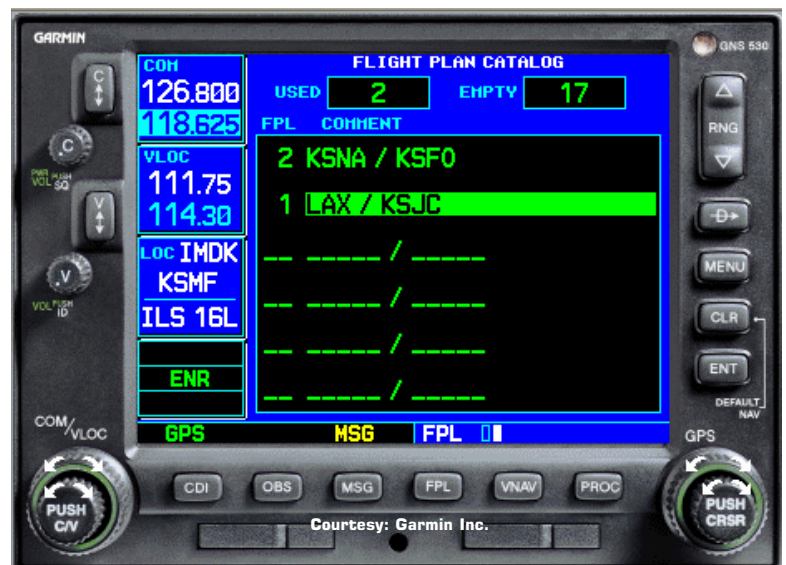
Figure 38. When returning from San Jose to the Southern California area, push FPL and twist the pull-turn knob once to open the "Flight Plan Catalog." Highlight your previous routing and press MENU.
