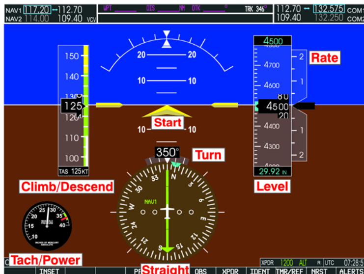
Figure 20. The primary instruments can be more easily identified by placing the names of the maneuver that they perform near that instrument on the PFD.
