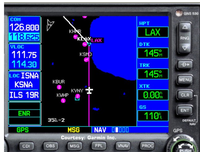
Figure 42. The routing above on Nav Page #2 indicates that you're enroute to LAX VOR.
