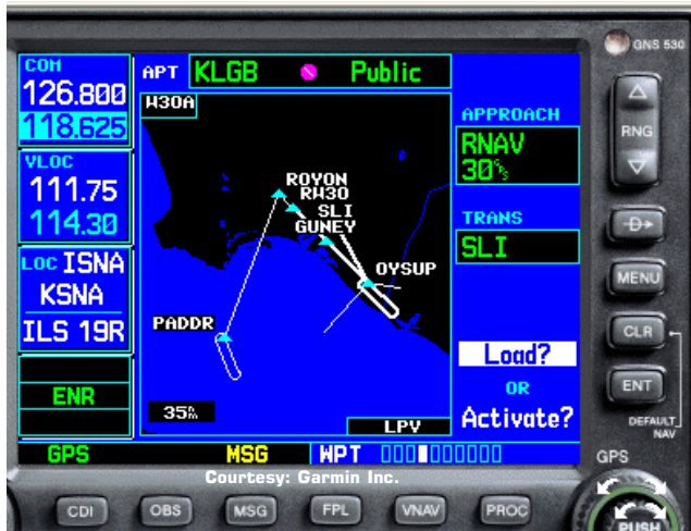
Figure 47. Select "Load" or "Activate" then press ENT. You should select "Load" here.
