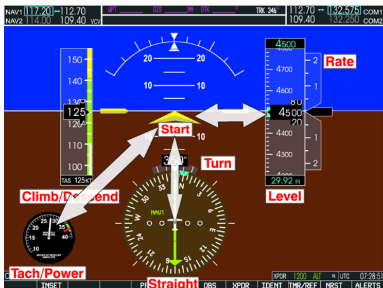
Figure 21. The scan above shows the primary instruments for straight and level flight.
