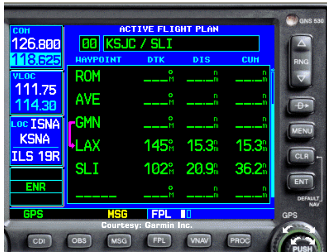
Figure 41. The SLI VOR has been added to the end of your routing past LAX VOR.
