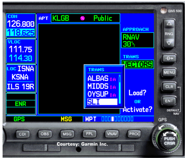
Figure 46. After pressing ENT, you are given the choice of approach transition. Scroll down to SLI and choose this option by pressing ENT.
