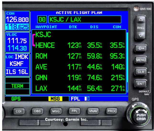
Figure 40. Your original flight plan from LAX VOR to San Jose airport has been inverted and the KSJC-HENCE leg activated.
