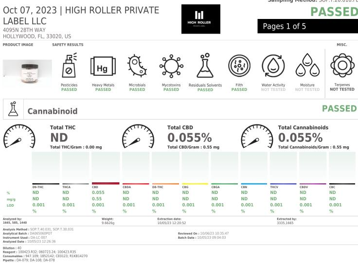
Full Sp um cannabinoid analysis utilizing High Performance Liquid Chromatography with UV detection in accordance with F.S. Rule 64ER20-39
