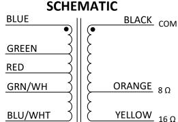
PRIMARY: 9.1K  $\Omega$  CT WITH +/- 25% ULTRA LINEAR TAPS SECONDARY: 8/16  $\Omega$ POWER: 35W
