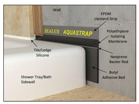
In roll format two siliconized release liners (1 & 2) cover the butyl adhesive bed. The upper release liner is a flexible and deformable 50 micron polyethylene skin that extends over both the 2mm thick adhesive bed and the 3mm round neoprene backer rod - without compressing the neoprene backer rod. The lower release liner is a non-stretchable paper that prevents installers stretching Aquastrap during the installation process.
