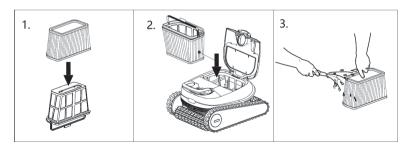
The filter paper core is a fragile part, which can filter particles below 100µm, and its service life is less than 72 hours. (The filter paper core can be used without affecting the performance of the robot, and it is strongly recommended that the filter paper core not beused in a dirty swimming pool. It is best to give final cleaning after majority of cleaning has been carried out)
