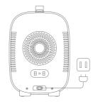
**Step2.**Connect the power interface on the back of the product to the household socket with the power cord.
