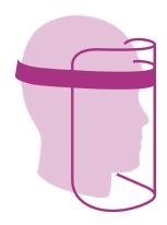
FS100 full length faceshields are made of flexible and shatterproof PET plastic. They are adjustable to fit the face and are held in place with an elastic head strap. These visors have an anti-fog membrane and a comfortable foam headband designed to protect the entire face.
