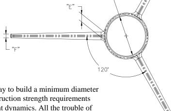
There's really no easier or faster way to build a minimum diameter rocket, and still maintain the construction strength requirements dictated by high power rocket flight dynamics. All the trouble of oversize airframe tubes, individual through-wall fins, centering rings, slotting, fin filleting, and the like are eliminated. The Acme fin canister simply slides onto your airframe tube, and epoxies into place.
