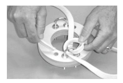
With the Kevlar cord, find and mark the center point. Take the finished c-ring assembly and with one end of the Kevlar cord, **LOOP AROUND AND THROUGH ONE U-BOLT** and continue by inserting through the 1/2" opening adjacent to that u-bolt. Pull several feet of the cord through that opening. Now take the other end of the Kevlar cord and repeat the same procedure with the other u-bolt, 1/2" opening and pull through until the center point on the cord is in-between the two u-bolts.
