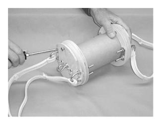
**DO NOT USE ANY EPOXY YET.** Place a witness mark from the 3.9"x 8" tube to the yet un-attached collar assembly so you can line up the collar properly when attaching it permanently.
