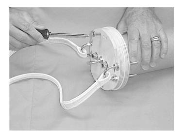
**DO NOT USE ANY EPOXY YET.** Slide the second collar assembly onto the opposite end of the 3.9"x 8" tube with the u-bolts again facing outward followed by the rounded corner endplate over the av-bay all-threads. Re-attach the av-bay wing nuts onto the all-threads and rotate the loose av-bay collar so you can attach and finger tighten the two machine screws through the rounded corner endplate into the inserts found in the mounting collar.
