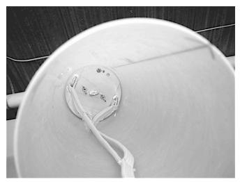
NEVER PERMANTLY MOUNT THE AV-BAY INSIDE OF THE HOLDER. It is designed to be removable for your ease of use. NEVER, EVER ATTACH YOUR RECOVERY HARNESS TO THE EYEBOLT ON THE ELECTRONICS BAY. THAT EYEBOLT IS ONLY A KNOB TO REMOVE THE TRAY AND CANNOT ACCEPT THE STRAIN OF RECOVERY EQUIPMENT ATTACHMENT. Instead, your recovery harnesses will connect to the Kevlar bridles.
