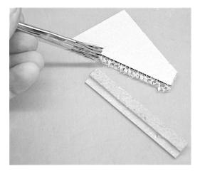
When completed, remove the tape and inspect your results. Check to see that both parts are firmly locked together and straight in line with each other. Notice the amount of excess epoxy that has migrated to the exposed area of the sample under the tape. Your goal is to use sufficient epoxy to bond the parts together, but minimize the amount squeezed out that you didn't wipe up prior to curing. Otherwise, some sanding may be necessary to remove hardened excess epoxy.
