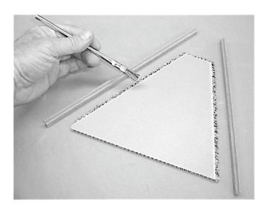
Apply epoxy in a similar method to your practice exercise above, wipe off excess epoxy, tape and allow curing. To speed up the process, you can apply edging in the same method to the opposite edge. **DO NOT APPLY EDGING TO THE FIN TIP UNTIL NOTIFIED.** Do this procedure to all the leading and trailing edges for the upper and lower fins. Set aside and allow curing flat on the wax paper surface.
