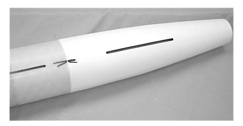
BE AWARE OF THESE MARKS, IT WILL BE NECESSARY TO LINE THEM UP WHEN PERMANENT ATTACHMENT TAKES PLACE LATER. DO NOT EPOXY THE MOTOR TUBE/TAILCONE ASSEMBLY OR COUPLER CENTERING RING INSIDE OF THE AIRFRAME YET!
