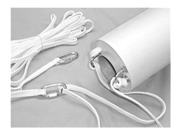
Locate the two 5/16" quick-links and 1/2" x 25' Kevlar shock loop. Insert a quick link through each loop end and attach one loop to the above 1/2" Kevlar between u-bolts that extends above the airframe coupler. The opposite end of the shock loop will eventually attach via 5/16" quick-link and the Kevlar bridle to the lower part of the av-bay located inside of the upper airframe.
