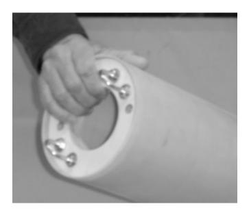
If satisfied, remove the c-ring assembly and loosen (not remove) the u-bolts so you can spread a thin layer of epoxy between the c-rings, tighten the u-bolts and confirm that the assembly will still slide inside of the coupler.
