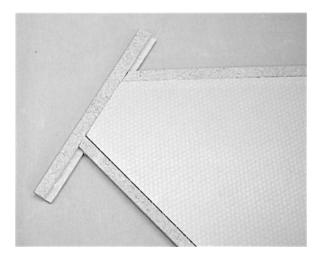
Now you can "flat sand" the faces of all the fins and edges **BEING CERTAIN NOT TO SAND INTO THE COMPOSITE FIN MATERIALS.** It will be necessary to fill the cavities left on the tip edging prior to shaping of the edging into airfoils.
