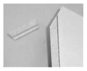
Take additional edging and apply in the same manner to the tips of all fins MAKING SURE THAT EXCESS EDGING EXTENDS PAST THE PREVIOUSLY MOUNTED LEADING AND TRAILING EDGING. When completed, trim and sand the excess edging in the same "line" as the previous edging.
