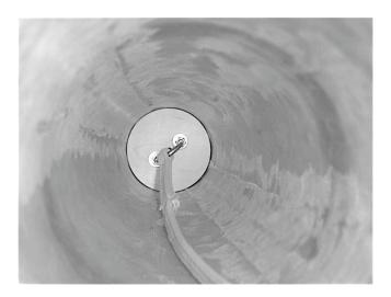
Using a 5/16" quick link, connect the loose end of the above Kevlar shock loop (with piston connected to the nose cone) to the Kevlar bridle found at the av-bay holder, 14"-15" inside of the upper airframe.
