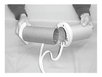
Line up the two holes in the endplate with the two inserts mounted in the collar assembly and install the two machine screws finger tight.
