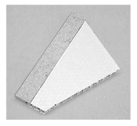
Now collect all the composite fins and edging material. Turn all the fins with the routed "channels" up on wax paper. YOU MUST APPLY EDGING TO THE LEADING AND TRAILING EDGES OF THE FINS FIRST! Take a section of the edging and with your Xacto (or equivalent) razor saw cut a piece 4" LONGER than the length of the fin edge you want to cover. THERE MUST BE THIS EXCESS EXTENDING ON BOTH ENDS OF THE FIN EDGE FOR A LATER STEP.
