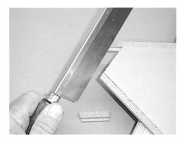
You will now do the same "trimming" to the opposite end of excess edging, down by the fin tabs. This procedure is slightly tricky as you must follow the fin tab "line".
