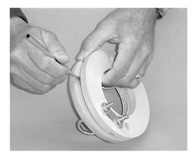
If not, loosen the u-bolts and adjust the c-rings until the assembly will fit inside the
