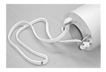
When the above assembly is finished, be sure all Kevlar cord is pulled tight inside of the airframe and all excess is outside.
