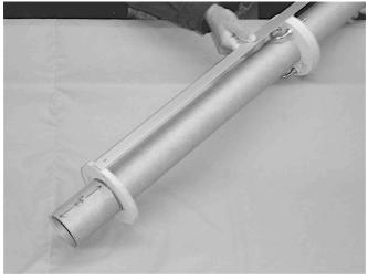
Apply a generous amount of epoxy onto the motor tube between the previously made marks. Push the centering ring into the ring of adhesive, and tape into place square to the motor tube, CHECKING ALIGNMENT OF THE SMALL HOLES TO THE UBOLTS BELOW, THAT THEY ARE IN A STRAIGHT LINE. Also be sure there are no epoxy runs. After epoxy has cured, apply epoxy fillets to both sides of this ring/body tube joint, set aside the entire assembly and allow curing.
