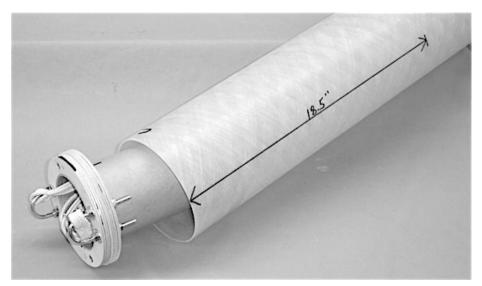
WITHOUT MOVING THE HOLDER, make a mark around the inside of the airframe next
