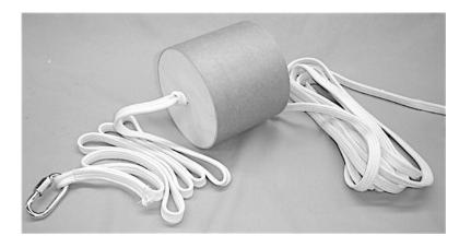
Locate the 3.9" bulkhead with loosely attached u-bolt. Remove the u-bolt and slip it through the above sewn Kevlar loop end found on the **LONGER SIDE** of the shock cord and permanently re-attach to the 3.9" bulkhead. Using that bulkhead, epoxy into the nosecone as far as it will go. Be certain to mount it well because should it fail, your nosecone will be lost. Do not allow epoxy to get on the Kevlar shock cord.
