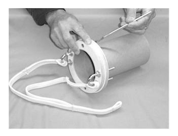
Find the av-bay kit and the two rounded corner plywood endplates. First, open the av-bay kit and remove the two larger body bulkheads and set aside. You will **NOT** use them. Instead the rounded corner endplates will be substituted. Assemble that kit per the included instructions so the rounded corner endplates are oriented the same direction on either end of the av-bay.
