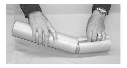
Now butt the extension to the 48" x 3" motor tube end opposite of the Slimline retainer. Slide the split coupler over the joint of the two tubes until the coupler is equal in length on both sides of the joint.
