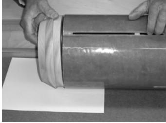
With a marking pen or pencil, draw a line/circle on the inside of the airframe where the rear-
