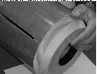
**CAREFULLY**, stand the entire assembly vertical, tailcone end down, BEING CERTAIN THE TAILCONE IS JOINED INSIDE THE BOTTOM OF THE AIRFRAME AND THE BOTTOM OF THE SLIMLINE IS FLUSH WITH THE BOTTOM OF THE TAILCONE.
