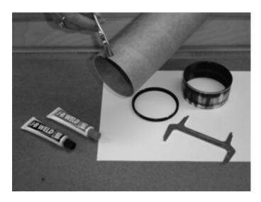
Next, locate the two 7.5"x 3.0" centering rings with four 5/16" and two 1" extra holes, two u-bolts with four each hex nuts and washers and one ½" Kevlar bridle with three sewn loops. WITHOUT BONDING THE CENTERING RINGS TOGETHER, begin by locating the "witness" marks on the sides of the centering rings and align them.
