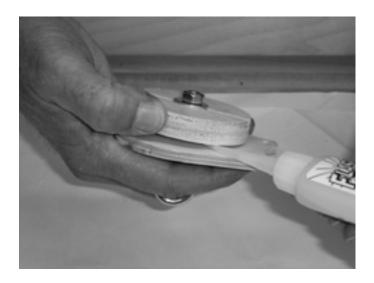
When finished, push both pieces together, **LINING UP THE DADO SLOT IN CORRECT POSITION**, and tighten the outside nut with Loctite or equivalent. IMMEDIATELY WIPE AWAY **ANY** ADHESIVE FROM THE OUTSIDE OF THE POD COVER ASSEMBLY. Continue this procedure with the remaining pod cover assemblies. After curing, check the fit of the pod cover assembly in position with the main av-bay assembly. If necessary, sand the edges of the bulkhead until it fits properly inside the av-bay pod.
