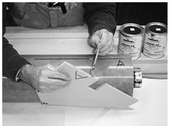
Insert this A fin into the A slot until the root edge presses against the motor tube and
