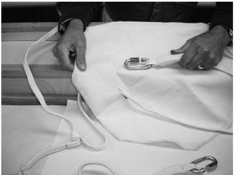
By putting the longer of the two included shock loops between the booster section and what will eventually be the upper airframe, you are insuring that during drogue descent, both sections of your Sledgehammer will be separated sufficiently to help prevent uncontrolled contact with resulting damage.
