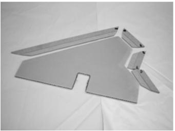
WITHOUT ADHESIVES, gently press each piece, **TONGUE FIRST**, into the correct **GROOVE** of the fin material. It is possible that some additional honeycomb material found in the fins may need to be removed allowing complete insertion of the edging tongue up to the point where the edging regains full thickness. It also may be necessary to adjust each piece side
