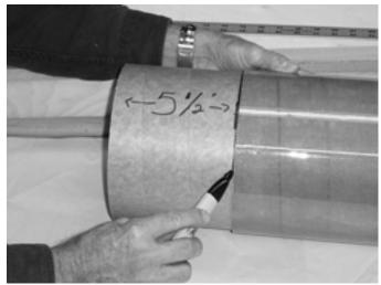
KEEPING THE COUPLER AT EXACTLY THAT POINT, temporarily apply masking tape to hold the coupler in position. With your marking pen AND WITHOUT MOVING THE COUPLER, mark the interior circumference of the Dyna-Wind airframe flush at the opposite end of the
