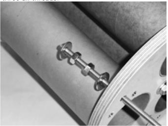
Without tightening any nuts or washers, continue insertion of the three all-threads through the first-top av-bay mounting ring and then through the three opposite 5/16" holes located EXACTLY ACROSS in the second-bottom av-bay mounting ring. Spin (or "run-up") all the nuts and washers that reside between the two av-bay mounting rings allowing all three all-threads **WITH NUTS ONLY FLUSH ON THE ENDS** to stop in contact with the "outside" of the top av-bay mounting ring.
