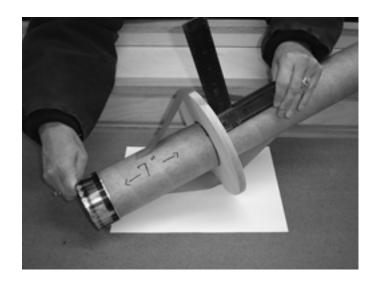
It is recommended you stand the motor tube on end PREVENTING any runs of epoxy down the tube. ALLOW THIS JOINT TO CURE WITH NO EPOXY RUNS ON THE TUBE OR "FLOW-OUT" ON THE CENTERING RING. FAILURE WILL CAUSE GREAT DIFFICULTY IN FOLLOWING STEPS. After curing of the above sub-assembly, place a mark on the end of the above motor tube, OPPOSITE the Slimline retainer, 6.5" down from the open end of the tube.
