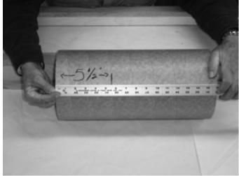
Temporarily (WITHOUT ADHESIVES) slide the coupler into one end of the  $7.5"x\ 30"$  Dyna-Wind airframe until the mark at 5.5" on the coupler is flush with one end of the airframe.
