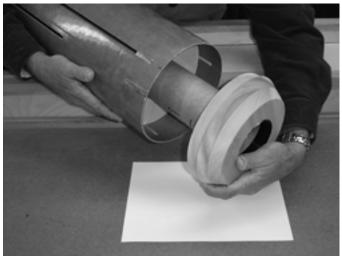
With the flat part of your hand, push both the motor tube and tailcone together further into the slotted 7.5" airframe **STOPPING** when the reduced diameter end of the tailcone has joined inside the bottom of the airframe (cone end of tailcone is still exposed) and THE VERY BOTTOM OF THE SLIMLINE IS FLUSH WITH THE VERY BOTTOM OF THE TAILCONE.
