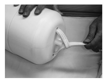
PLEASE DO NOT UTILIZE THE ATTACHMENT LUGS MOLDED INTO THE BASE OF THE NOSECONE. Often, those attachments cannot handle the strain and will break free of the rocket "assembly" during ejection.
