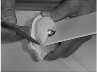
Without removing the av-bay board from the pod cover assembly **AND STILL USING NO ADHESIVES**, slip the opposite end of the board into the dado slot of one of the remaining 2.5"x 1/2" bulkheads, confirming "fitment" and that the board "width" does not extend past the outside of the bulkhead.
