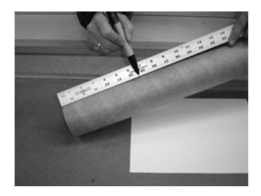
WITHOUT ADHESIVES, locate the 7.5" centering ring assembly with two u-bolts and Kevlar bridle and slide onto the same end of the tube (side with Kevlar bridle facing away from the Slimline end) until the wood of the BOTTOM (facing the Slimline retainer) CENTERING RING IS EVEN WITH THE JUST MADE MARK 6.5" down on the tube.
