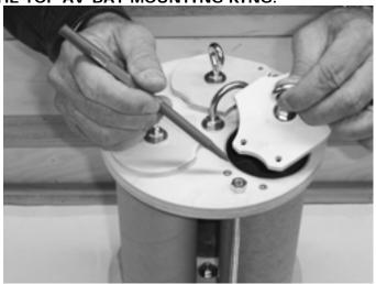
If they do not, it will be necessary to disassemble the pod cover assembly and FLIP the pod cover over so it will. REMEMBER TO KEEP THE BULKHEAD WITH DADO SLOT AND THE POD COVER ARRANGED AS SHOWN ABOVE TO POSITION THE DADO SLOT PROPERLY. Once you are satisfied, loosen the outside nut to allow a small gap between the pod cover and bulkhead with dado slot. Squirt a small amount of THICK CA GLUE around the perimeter of the bulkhead and the pod cover.
