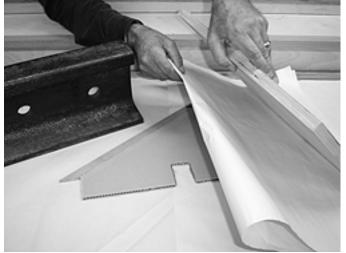
Carefully, without shifting, lay a solid-weighted object on top to provide downward pressure on the curing fin/edging. IT IS VERY IMPORTANT THAT HEAVY DOWNWARD PRESSURE BE APPLIED DURING CURING AS THIS WILL PRODUCE A BETTER, FINAL PRODUCT.
