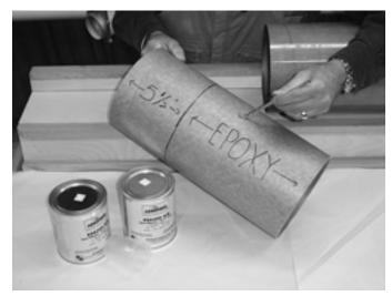
Slowly insert the epoxied coupler end into the epoxied 7.5" airframe end. USE A TWISTING MOTION as the coupler is inserted slowly into the airframe. HINT: KEEP THE COUPLER/AIRFRAME LEVEL TO SLIGHTLY LOWER WITH THE OPPOSITE END.
