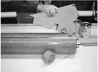
Inspect the epoxy that was left on the motor tube to confirm you have a complete "footprint" along the length of the root edge. USING FILLERS WITH EPOXY WILL HELP PREVENT "RUNS" OF EPOXY AROUND THE MOTOR TUBE WHICH WILL CREATE GREAT PROBLEMS DURING ATTACHMENT OF FINS B AND C.
