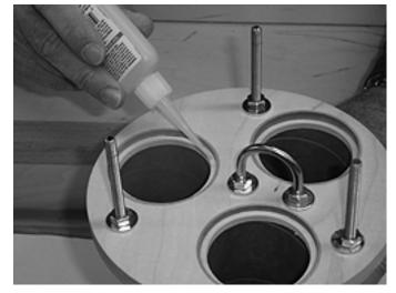
Finally invert the entire Triad av-bay assembly and insert the remaining six 8/32 machine screws and washers through the holes located in the pod covers, thread into the brass inserts located directly beneath.
