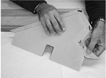
Continue the dry fitting for all three fins. Once satisfied with the "fitment", remove all the edging and arrange around the perimeter of the fins, **WITHOUT COMPROMISING THE CORRECT ORDER.**
