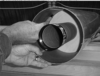
After making the "positioning marks", carefully remove the motor tube assembly from the airframe and set-aside. With sandpaper, "scuff" the interior of the airframe just above the rear-most mark/circle and just below the upper most mark/circle.
