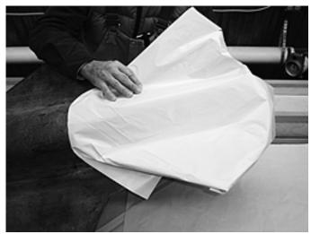
Remove the paper and cut out the indicated shape to create a cloth reinforcement pattern.
