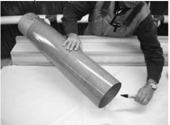
Mix sufficient 30minute epoxy (or longer cure) to apply a thin coat to the 11.5" exterior of the coupler (NOT THE 5.5" AREA) and to the interior of the Dyna-Wind airframe where that 11.5" section of coupler will permanently reside. Using an old credit card or similar material, spread an even coat over these areas. **DO NOT SPREAD EPOXY OVER THE 5.5" SECTION OF COUPLER OR PAST THE 11.5" MARK MADE INSIDE THE 7.5" DYNA-WIND AIRFRAME.**
