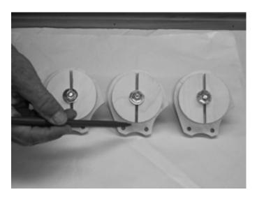
WITHOUT ANY ADHESIVES, drop all three pod cover assemblies into position on the av-bay where the brass-threaded inserts are visible. TURNING ALL POD COVERS AS NECESSARY, CONFIRM THAT THE TWO SMALL HOLES DRILLED IN THE POD COVERS LINE UP WITH THE MATCHING BRASS-THREADED INSERTS LOCATED IN THE OUTSIDE OF THE TOP AV-BAY MOUNTING RING.
