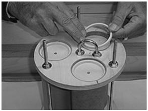
Push each centering ring and 'o' ring in until it comes in contact with the bottom of the removable pod insert. **BE CERTAIN THE POD INSERTS HAVE NOT BEEN PUSHED OUT OF THE POD CONTAINERS!**
