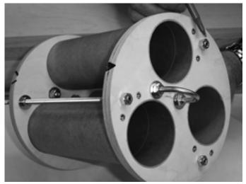
Before going further, thread first a washer and then a nut onto the three exposed ends located on the "outside" of the bottom av-bay mounting ring. DO NOT TIGHTEN as you are
