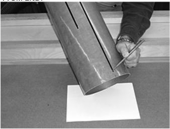
In a later section of these instructions, you will be inserting three identical fins in those slots. Further up the same airframe are two longer slots where later you will be inserting two identical wings. BE AWARE OF THE DIFFERENT POSITIONING AND LENGTH OF THESE FIVE SLOTS.
