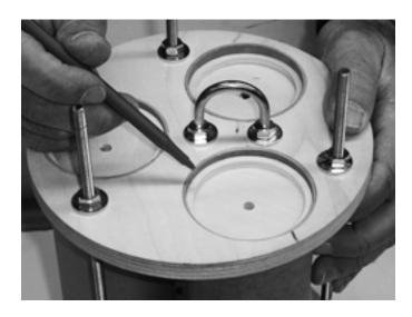
After checking "fitment", remove all three pod inserts and 'o' rings leaving the centering rings UN-MOVED. CAREFULLY, with THIN CA glue, wick the adhesive around the three centering rings **BEING CERTAIN THE ADHESIVE HAS NOT MIGRATED AWAY FROM THAT LOCATION.** Leave open and allow curing prior to replacement of the 'o' rings and pod inserts.
