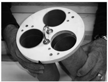
IT IS CRITICAL THAT ALL THREE TUBES ARE FLUSH/SQUARE ON THE ENDS AND STRAIGHT WITH ONE ANOTHER AND THE U-BOLT FACING OUT. DO NOT ALLOW ANY EPOXY TO MIGRATE INSIDE THE TUBES. Set aside to cure with tubes vertical.
