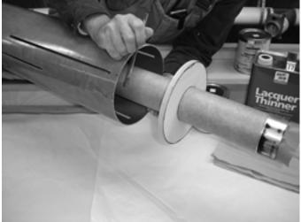
Be sure the Kevlar bridle is "stuffed" inside the motor tube to keep it out of the way. In addition, apply masking tape to the interior of the Slimline motor retainer to prevent accidental epoxy contact.
