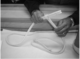
Mount a second 5/16" quick link to the free end of the 44" shock cord.
