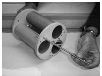
Next thread first a washer and a nut AND THEN A SECOND NUT AND WASHER **IN THAT ORDER** onto all three all threads.
