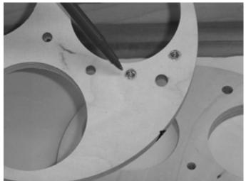
Begin by putting one nut first and then one washer on each "leg" of the two u-bolts, running the nuts and washers to the very top. With both av-bay mounting rings temporarily placed together, match witness marks on the edges. KEEP THOSE MARKS ALIGNED THROUGH-OUT THIS ASSEMBLY.
