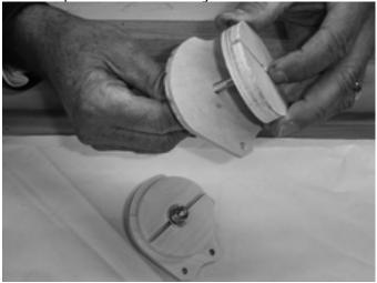
Referring to the following photograph, notice the position of the dado slot to the pod cover. IT IS HIGHLY RECOMMEND THAT ALL THREE POD COVER ASSEMBLIES ARE BUILT IN THIS MANNER.
