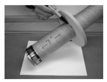
Upon completion, temporarily slide the single centering ring several inches back up the tube away from the just marked area. With sand paper, scuff the motor tube in that area to abrade the surface but leaving your marks.
