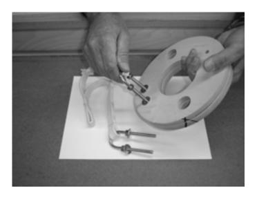
Turn over the centering rings and place one washer and one nut onto each leg of both ubolts and lightly finger tighten.
