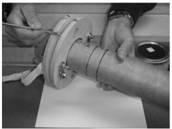
BEFORE THAT EPOXY HAS TIME TO CURE, place a generous amount of epoxy between the two lines and slide the centering ring assembly (side with Kevlar bridle goes on last) onto the tube between the marks.
