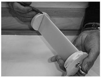
Once you are satisfied with the "dry-fit", mix sufficient epoxy to apply in the dado slot of POD COVER ASSEMBLY AND THE NOTCHED END OF THE AV-BAY BOARD and join together. Wipe away any excess epoxy and confirm that the av-bay board does not extend outside of the dado slot. REMEMBER, WIPE AWAY ANY EXCESS EPOXY. Once assembled, stand on end and allow to cure.
