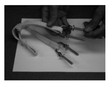
Next thread onto and run up ONE hex nut and washer on all four legs of both u-bolts; run the nuts to the very top of the threads. Insert both u-bolts into the four 5/16" diameter holes located in the centering rings (keeping the witness marks together) with both u-bolts facing the same direction (and the Kevlar bridle on the same side). Avoid having twists in the Kevlar bridle.
