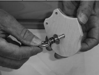
Insert that eyebolt through first the sculpted pod cover and then through the 2.5"x1/2" bulkhead leaving the dado slot in that bulkhead FACING OUT. Thread a second washer first and then nut onto the exposed end of the eyebolt FINGER-TIGHT ONLY.
