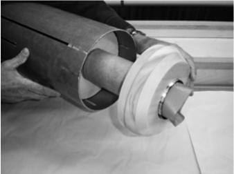
YOU CANNOT, CANNOT ALLOW ANY AMOUNT OF ADHESIVE TO BE ANYWHERE ON THE INSIDE REAR FIVE INCHES OF THE AIRFRAME.
