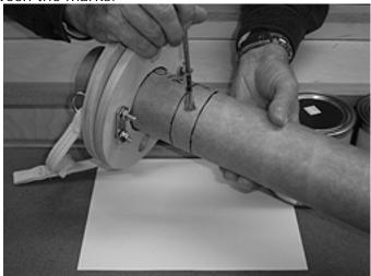
Once in position, SECURELY TIGHTEN ALL FOUR NUTS ON BOTH U-BOLTS.
