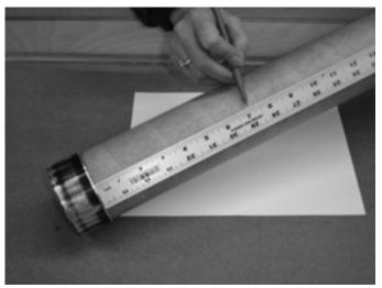
Take the single 7.5"x 3.0 centering ring, NOT THE CENTERING RING ASSEMBLY JUST ASSEMBLED, and slide that single ring onto the tube from the end opposite of the just attached Slimline body. Bring that ring (WITHOUT ANY ADHESIVE YET) down until it sits ABOVE the just made mark on the motor tube. With the centering ring square and perpendicular to the body tube, take a marking pen and make a circular mark on the motor tube on both sides of the centering ring.
