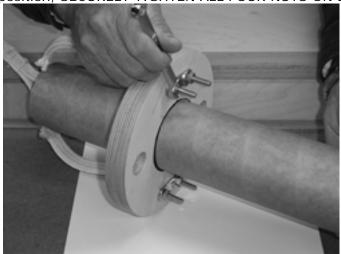
BE CERTAIN THIS ASSEMBLY IS IN POSITION ON THE TUBE, BETWEEN THE MARKS, "SQUARE AND PERPENDICULAR" TO THE MOTOR TUBE.
