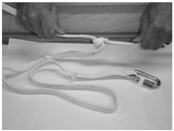
Next, slip a Kevlar chute pad over the still loose end (of the 25' shock-cord) and finally attach via a third 5/16" quick link to the Kevlar bridle located in the top of the lower booster section.
