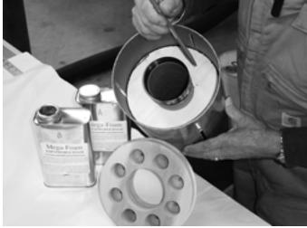
YOU CANNOT HAVE THE TWO PART FOAM RISE UP INTO THE AREA REQUIRED TO MOUNT THE TAILCONE. Remove the tailcone and mix a minimal amount of two part expanding foam, stir and pour evenly into this area and allow to "foam-up". BE CERTAIN
