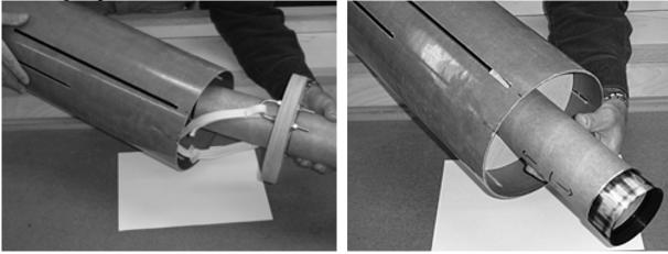
Next, slide the wood tailcone over the exposed-attached to motor tube Slimline retainer and stop.
