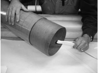
Holding the same shock cord end, thread it through one of the 1/2" drilled holes in the base of the nosecone and out the other drilled hole, threading it back upon itself as shown in the photograph.
