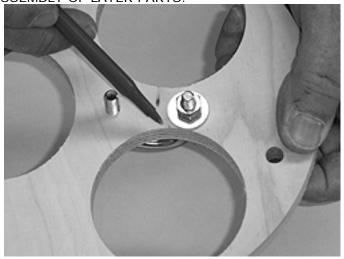
First, locate the two av-bay mounting rings with three 2.5" holes in each, two u-bolts and eight ¼" nuts with washers. Notice one of the av-bay mounting rings has six brass-threaded inserts; that mounting ring is the "top" of the completed Triad bay with the side showing six brass inserts closest to the surface to be considered the "out" side of that mounting ring.
