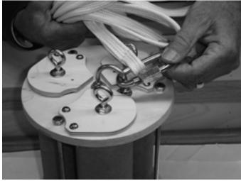
Thread the opposite loop first through one "looped end" of the short (44") Kevlar Shock Loop and tie into place over that short shock-loop with one simple overhand knot approximately FIVE FEET from the Triad av-bay.
