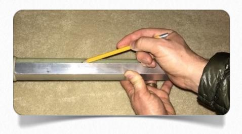
3. Lightly sand the attachment points on the airframe as well as the GLR Rail Guides for good adhesion. Mix J.B. Weld and attach first the GLR Rail Guide to the points on the airframe (see photo). While curing, sight down the tube to check for good alignment. It is also a good idea to place some tape on the GLR Rail Guides lightly securing them to the airframe. The tape will prevent a "drooping" of the GLR Rail Guide system as the J.B. Weld sets.
