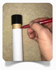
made at the ½" mark, draw a line around the motor tube.
