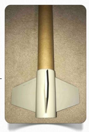
as you go, until the Aft edge of the GLR Acme Fincan lines up exactly with the Aft edge of the Airframe. Note: the tapered edge of the GLR Acme Fincan is Forward for aerodynamics. GLR Acme Fincan equals perfect alignment and ease every time!
