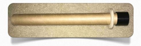
deploys and JB Weld is significantly stronger. Slide the Aft Centering Ring onto the motor tube, twisting as you seat it. Make sure that the Aft Centering Ring is level and parallel to the forward opening of the motor tube. Allow the JB weld to cure completely.
