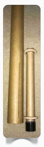
ing Ring will be Forward of the fin slots. On the outside of the airframe make a mark with a pencil where the Forward Centering Ring is and where the Aft Centering Ring is.
