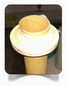
of GLR Aeropoxy. Add to this mixture GLR Glass-Micro-Spheres until you obtain a thick peanut buttery consistency. The ratio is typically 2 parts GLR Glass-Micro-Spheres to 1 part GLR Aeropoxy. More important that the ratio however, is the thick peanut buttery consistency. Create a large fillet between the motor tube and the Centering Rings by placing a liberal amount of material on both the Forward and Aft surfaces of the Centering Rings and al-
