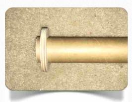
place the Forward Centering Ring. Place the Forward Centering Ring onto the motor tube. Measure from the Forward end of the motor tube (the end that is OPPOSITE the GLR Slimline Retainer attached) ½" and place a mark. Using a piece of paper wrapped around the motor tube, centered on the mark that you made at the ½" mark, draw a line around the motor tube.
