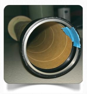
epoxy!) and apply it to the aft end of the motor tube, to the pencil mark of the motor tube. Then, install the GLR Slimline Motor Retainer onto the motor
