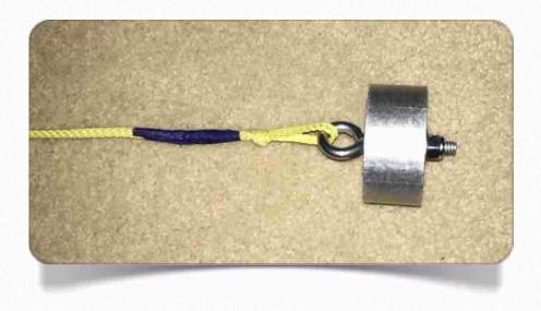
The GLR Hardpoint is now ready to be inserted into the airframe and test fit it. Hold the GLR Kevlar® shock cord and slide the GLR Hardpoint in and out of the airframe. You will want to insert the GLR Hardpoint from the Forward
