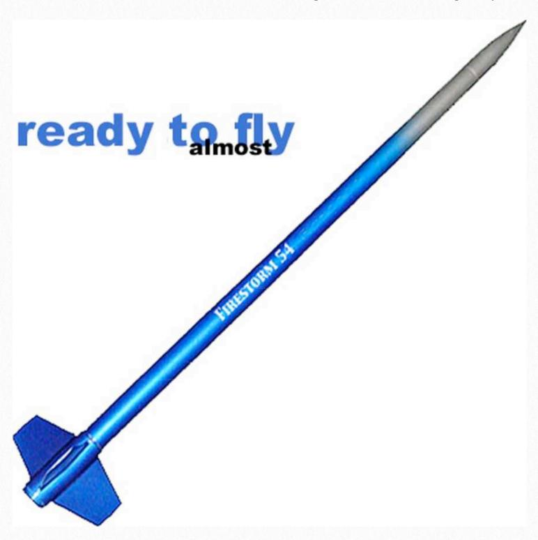
The FIRESTORM 54 is a perfect rocket for a level 2, duel deploy launch. The FIRESTORM is a 54mm minimum diameter rocket. This means that the airframe is the motor mount tube as well. The FIRESTORM is versatile as well: you can fly FIRESTORM as a single OR duel deploy rocket. Flying as a duel deploy typically allows the rocket to descend until the last few hundred feet, at which time a second para-
