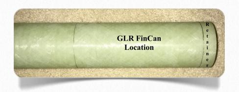
4. Remove both the GLR Slimline Motor Retainer and the GLR Acme FinCan from the body tube and set them aside. Mix some J.B.Weld (and only J.B. Weld - - don't use epoxy!) and apply it to the aft end of the tube, but do not go past the pencil mark for the GLR Slimline Motor Retainer. Then, install the GLR Slimline Motor Retainer on the tube. Turn the GLR Slimline Motor Retainer while you are in-
