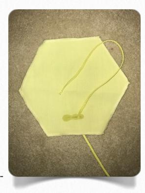
a result of the ejection charge deploying your recovery system when your rocket reaches apogee. We also provide a second GLR Kevlar® Parachute Heart Shield to protect the Main recovery system during the second deployment.
