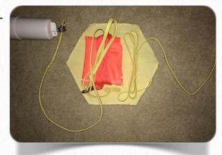
parachutes into their respective airframe. Begin with the Main parachute. Insert most of the GLR Kevlar® Shock Cord into the airframe first. Do this by creating accordion lengths of cord about 3-4" long, then insert into the tube. Leave about 3-4 feet of cord out.
