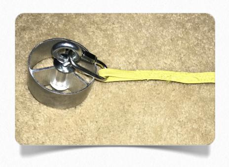
1/8" quick connect. Because Giant Leap Rocketry provides heat-resistant GLR Kevlar® Shock Cord in this kit, rather than nylon, there is no need to wrap the GLR Kevlar® Shock Cord with masking tape.
