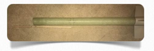
the FORWARD opening of the AFT airframe UNTIL THE LINE ON THE END YOU ARE HOLDING IS FLUSH WITH THE FORWARD END OF THE AIRFRAME (the end OPPOSITE the GLR Acme FinCan). Apply J.B. Weld in a ring to the interior of the airframe. The ring of J.B. Weld should coat the internal circumference of the airframe from the 11" to
