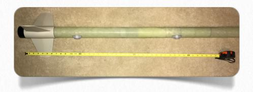
The tape will prevent a "drooping" of the guide system as the J.B. Weld sets.
