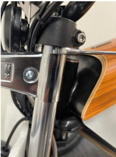
B. Tighten and secure the ears using a 4mm Allen wrench on the outside and a 10mm wrench inside.
