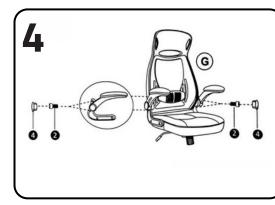
Place backrest between the mounting brackets (G>F). Screw in place with the dedicated screws and caps.
