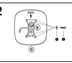
Turn the seat and assemble the leaning mechanism (E>D). Be ware of the direction.
