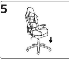
Turn chair. Place on top of the gaslift using the dedicated hole within the leaning mechanism.
