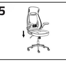
Connect the top to the base with the dedicated hole within the leaning mechanism.
