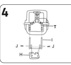
Place the feet support in the dedicated mounts by removing the two rubber rings (T). Slide the the brackets (I) through the plastic mount and roll the rubber rings back on. Attach pillow to brackets if not already pre-mounted.
