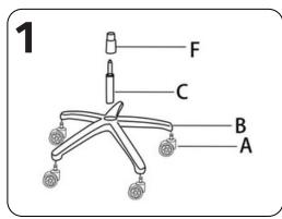
inside the middle of the base (C>B). Place the cover over the gaslift (F>C).
