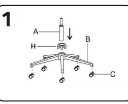
Attach all five casters **(C>B)**. PLace metal cover over the base **(H>B)**. Place the gaslift inside the middle of the base **(A>B)**.
