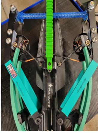
ALWAYS MAKE SURE BOTH PRESS ARMS ARE MOUNTED OVER THE SHINY ROUND PART OF THE BOLT. NOT OVER THE BOLT THREADS. IF MOUNTED CORRECTLY THREADS SHOULD BE EVEN WITH NUT EARS.
