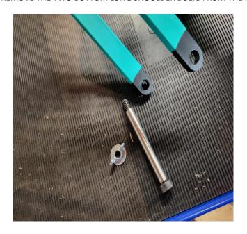
SLIDE BOTH PRESS ARMS OVER TOP AND BOTTOM LIMBS AND LOCATE THEM OVER THE TWO MOUNTING HOLES ON THE CROSSBOW. NEXT SECURE THE PRESS TO THE CROSSBOW WITH THE TWO LONG SHOULDER BOLTS YOU REMOVED IN THE PREVIOUS STEP
