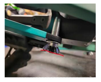
SLOWLY TURN THE PRESS KNOB TO COMPRESS THE LIMBS. NEVER COMPRESS IT MORE THEN NEEDED. JUST ENOUGH TO REMOVE THE STRING AND CABLES.
