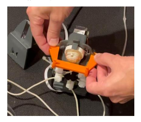
Make sure the bracket is pushed all the way down and resting the top of the two round solenoid housings:
