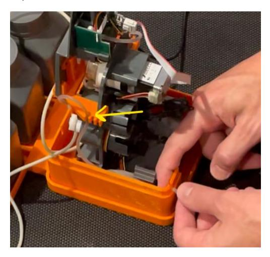
12) Feed the 3 reagent hoses through their slots in the front of the base. You can shorten them some by coiling extra cable through the slots in the bracket, see yellow arrows. Don't bend the hose too tightly or it will kink! :
