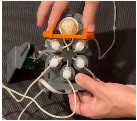
4) Get the base 3D printed part and insert the bigger Trident part, the two 'feet' sticking out of the bottom go into the two holes in the base. Make sure no cables or hoses are pinched between the base:
