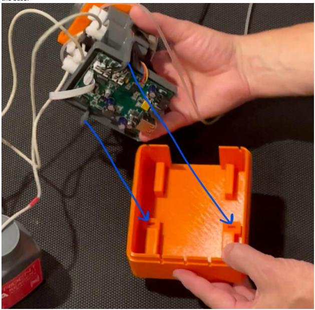
6) Use the clip part to snap the Trident board into the base:
