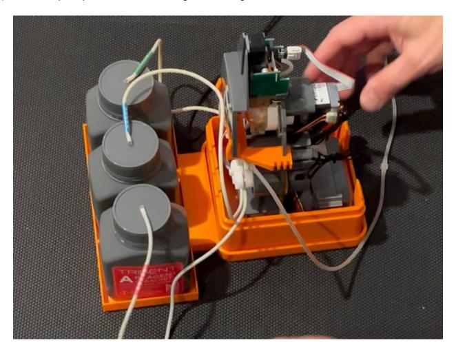
10) Feed the clear waste tube and black feed tube through the slots in the back of the base. Make sure the hoses are pushed down as far as they will go. If you want to shorten the hoses you can loop them up and gently tuck them under the clip. Be very careful to not cause any kinks or pinches in the hose! It is helpful to pass the hose through one of the slots in the 'bracket', see the yellow arrow:
