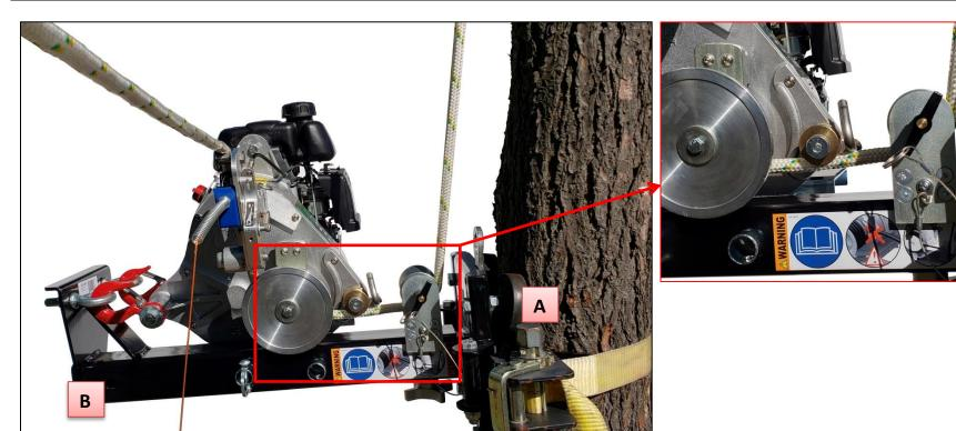
ATTENTION DO NOT GO OVER THE ROPE ENTRY PULLEY OF THE WINCH WITH THE ROPE AS IT WILL CREATE FRICTION AND WILL REDUCE LIFTING CAPACITY. GO UNDER THE ROPE ENTRY PULLEY OF THE WINCH. IN THIS CASE, THE ROPE ENTRY PULLEY OF THE WINCH WILL NOT BE USED.
