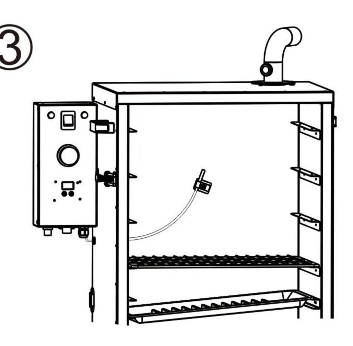
4. Put in the oil guide tray, then put in the oil guide basin (aims at the oil outlet of oil guide tray)
