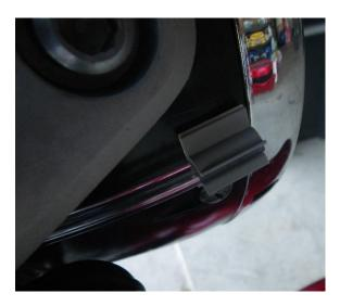
d. Route the opposite end of the inlet tubing to the reservoir location. Ensure that the tubing stays clear of engine components that could cause damage due to excessive heat and that the tubing will not be pinched when any removed components are replaced.
