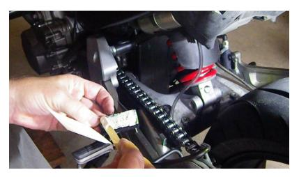
h. Press the chain applicator onto the swing arm slider within 5 minutes of applying the adhesive, ensuring that the applicator covers the entire width of the swing arm slider to ensure full contact with the chain.
