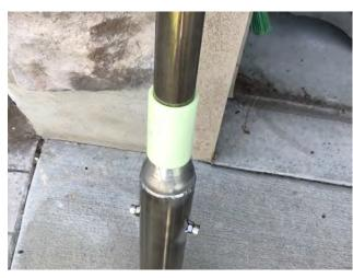
Insert the nylon spacer over the smaller end of the adapter. Depending on the size of your sleeve, the included nylon space can be used to ensure a snug fit. In some cases, the nylon spacer will not be needed.
