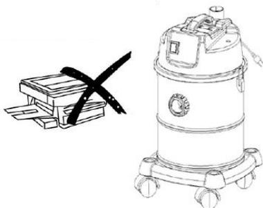
Do not overturn the machine in case water goes into and damages the motor.
