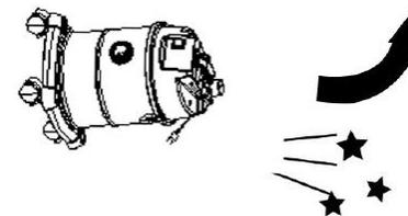
**Warning:** If water is emitted from the blower outlet, do not overturn the machine when repairing as water may get into and damage the motor.
