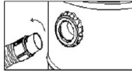
To use the blowing function, insert the hose connector into the blower outlet, make sure it is securely fastened.
