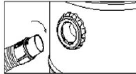
To remove the vacuum hose from the machine, press the release button on the hose connector and pull the connector out.
