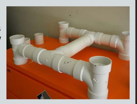
NOTE: There is no prohibition against gluing the PVC together; however, once glued together it will not easily fit into the Job Box for storage and transport. It is recommended that the cross pipe not be glued for easier storage.
